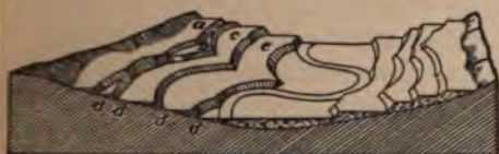
FIG. 172. — Schematic representation of a series of river terraces. a, b, c, e , successive terraces in order of age. d, d, d, d , terrace slopes formed of meander scars.
